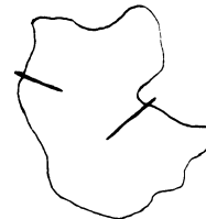
Fiber protrusion <0.5 micrometer
