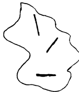
No fiber protrusion
